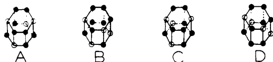
Figure 6. The possible site symmetries for \text{Eu}^{3+} ions located in site I: (A) D_{2h} ; (B) C_{2v} ; (C) C_s ; (D) C_{2h} , where \bullet denotes Si and \circ denotes Al. Note that only B and C possess the correct symmetry to account for the observed spectra. The europium ions located within the hexagonal prisms have been omitted for clarity.
